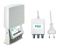
3-input (III+DAB, UHF, UHF) mast amplifier with 40dB gain and up to 116dBµV output level on UHF band, separate VHF/UHF amplification with independent gain adjustment (0-15dB) for each input and low noise figure. T2 technology with UHF cut band for LTE 4G @790MHz and 5G @694MHz. Power supply included in the package.
